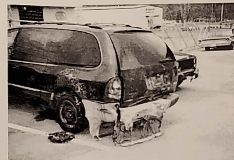
Results of a static electricity fire.
